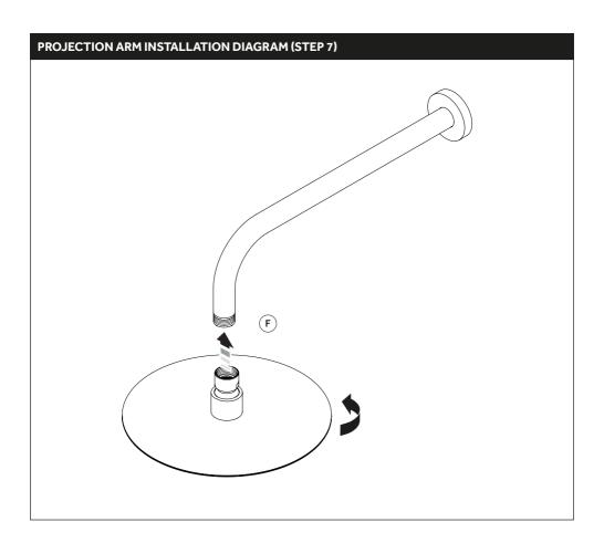
7. Flush all pipework and check for leaks before screwing the shower head onto the threaded end of the projection arm (F).
